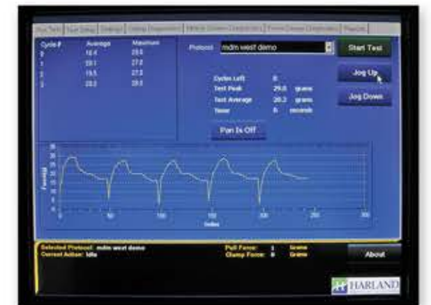
Test results are summarized in both tabular and graphic form as the test proceeds.
