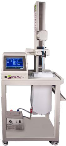
*Friction test system to measure lubricity*
